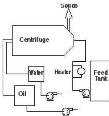
Figure 1 Flow Diagram for Three-Phase Centrifuge Process
